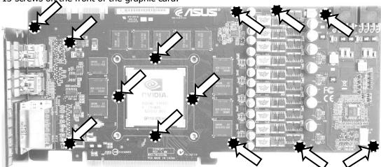
2. CLEANING THE PCB. Carefully detach the original heat sink after removing <u>all</u> fasteners securing it to the board and bracket. Wipe off the remains (by using non–abrasive cloth or Q-tip, as shown on sample photo) of the original thermal compound until the components and circuit board are completely clean. EKWB does not recommend using any liquids for removing paste.
