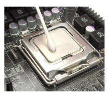
3. APPLYING THERMAL COMPOUND. Apply thermal compound: lightly coat nVidia GF110 GPU chip with for example Arctic Cooling MX-2  $^{\text{TM}}$  or MX-4  $^{\text{TM}}$  thermal grease. EKWB recommends to apply thermal grease in cross form for best performance (see sample picture).
