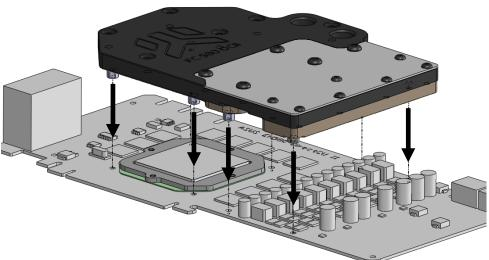
5. ATTACHING BLOCK TO GRAPHIC CARD. By using Philips screwdriver screw in enclosed M3x4 DIN7985 screws. EKWB recommends start screwing the screws around the GPU core and continue outwards.
