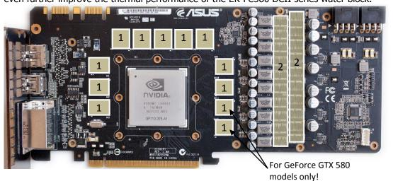
2. PLACING GPU REINFORCE PLATE ON PCB. Place metal reinforce and washer on PCB as shown on picture below and screw it in with enclosed M3x4 screws. Please use encased PVC washers under each screw. Make sure you use fasten screws equally and do not use too much force.
