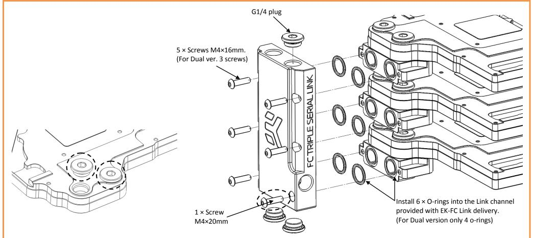
Plug both G1/4 ports on copper with encircled EK-Plug G1/4. Use Allen key to tighten the plug.
