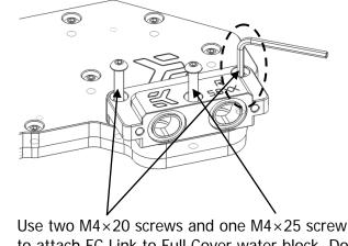
to attach FC Link to Full Cover water block. Do not use high force when tightening.
