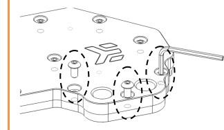
Unscrew three encircled M4×8mm screws with enclosed 2,5mm Allen key.
