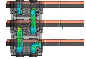
Serial or successive flow: Water starts flowing initially through first block, continues to second block and ends up with the third block.
