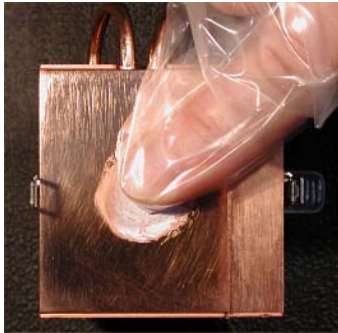
Picture 4: Applying compound on water block.
