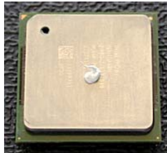
Picture 5: Applying compound on processor.
